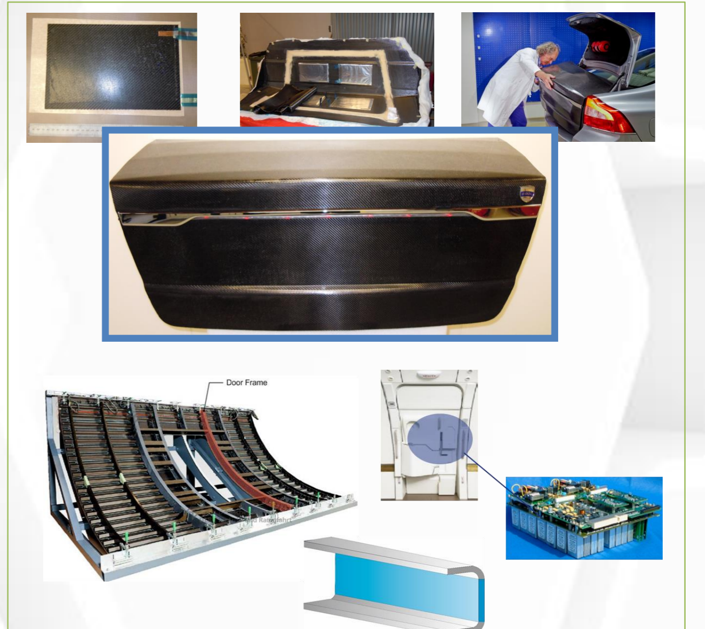
(Top) Volvo S80 composite bootlid with four stacks of four structural supercapacitors within; (Bottom) fuselage C-beam multifunctional demonstrator replacing supercapacitor bank
