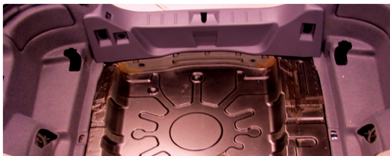
Volvo car spare-wheel floor to be replaced with structural energy storage material in the STORAGE project
