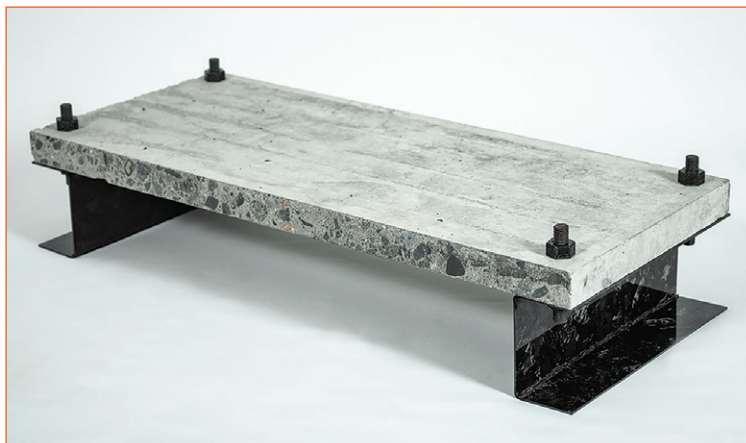
Fig.1: Firmly support concrete block with CFRTP bolts and plates
